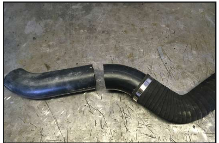
Saw part of the rear air duct as the sample
