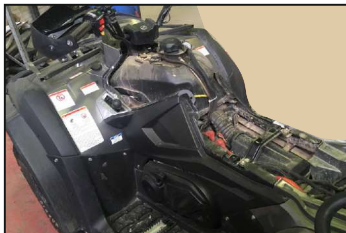
Remove the seat and fuel tank panel
