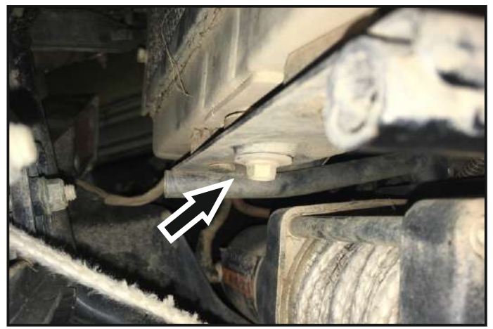
Unscrew the radiator mount bolt
