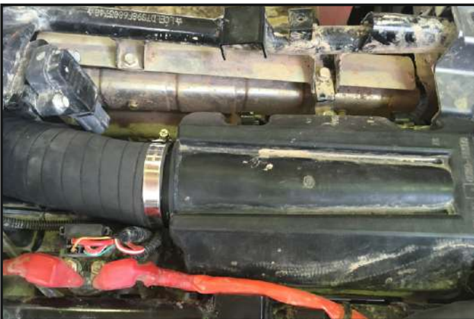
Install the adapter to the air filter housing
