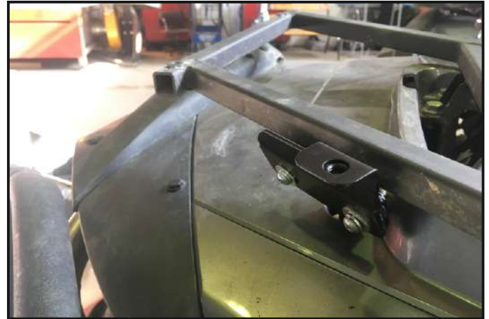
install the housing brackets of relocation box
