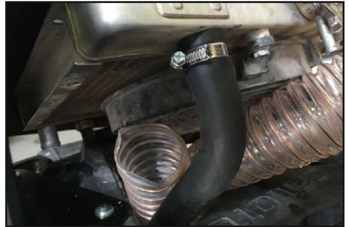
Install the bent hose on the radiator
