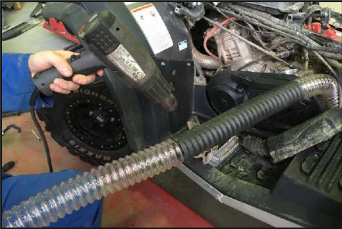
Install heat shrink tube along the engine
