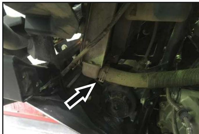
Remove the hose. Drain the antifreeze
