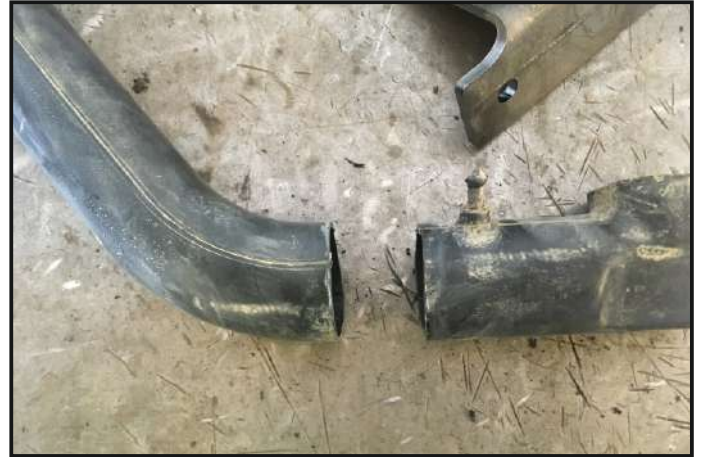
Saw part of the rear air intake tube as the sample
